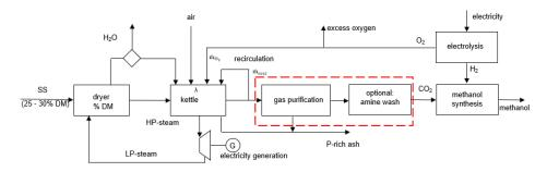
A simulation software (Aspen Plus) is used to model the oxyfuel combustion of sewage sludge and subsequent flue gas treatment on a pilot scale. Two configurations are investigated:
